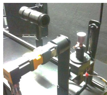
Figure 2 The goniophotometer for the measurement of the luminous intensity distribution of the lamps.
