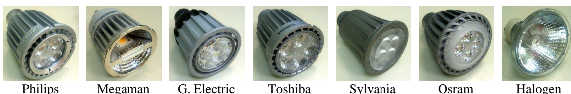
Figure 1 Photographs of the tested LED lamps and a typical Halogen reflector lamp.
