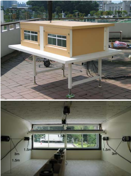
Figure 3 View of measurement in scale model
