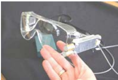
c/o Lighting Research Center Figure 4 Prototype of the LRC's circadian dosimeter, the "Daysimeter".
