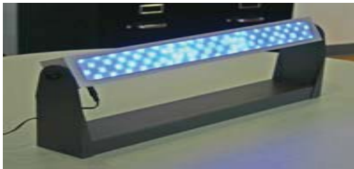
Figure 3 The LRC designed the luminaires for the study using LEDs
